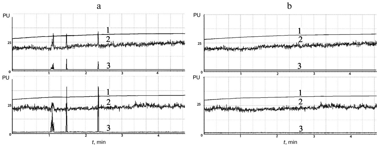
Fig. 3. An example of simultaneous recordings from two analyzers: a) with motion-induced noise; b) after filtering out the noise. 1) Temperature; 2) LDF-gram; 3) motion sensor recordings.
