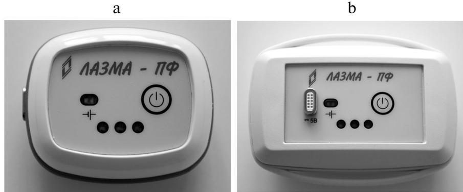
**Fig. 1.** LAZMA PF wearable analyzer modifications: a) for monitoring microhemodynamics (LDF); b) for monitoring both microhemodynamics (LDF) and oxidative metabolism (FS).
